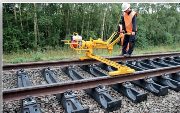
KLP® Hybrid Polymer Track Sleepers, Zwolle (The Netherlands).
